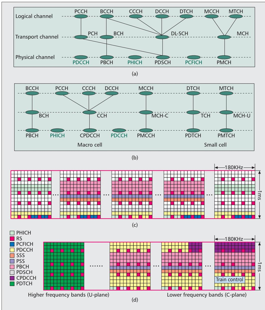
**Figure 3.** Channel mappings and frame structure: a) channel mappings in conventional LTE networks; b) newly redesigned channel mappings; c) frame structure in conventional LTE networks; d) newly redesigned frame structure.
