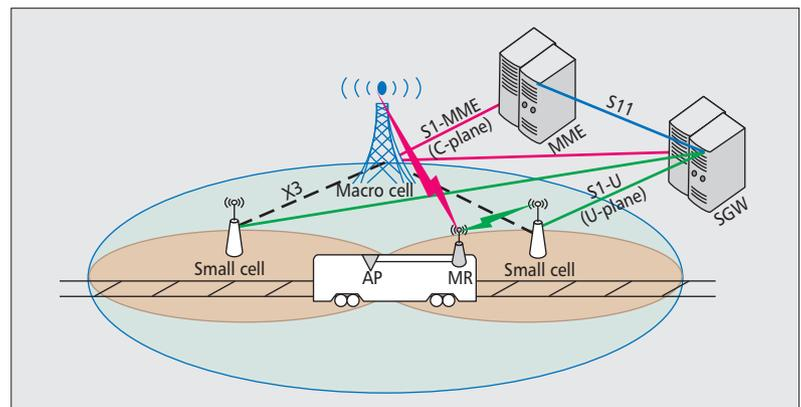
**Figure 1.** The C/U-plane decouple architecture for railway wireless networks.
