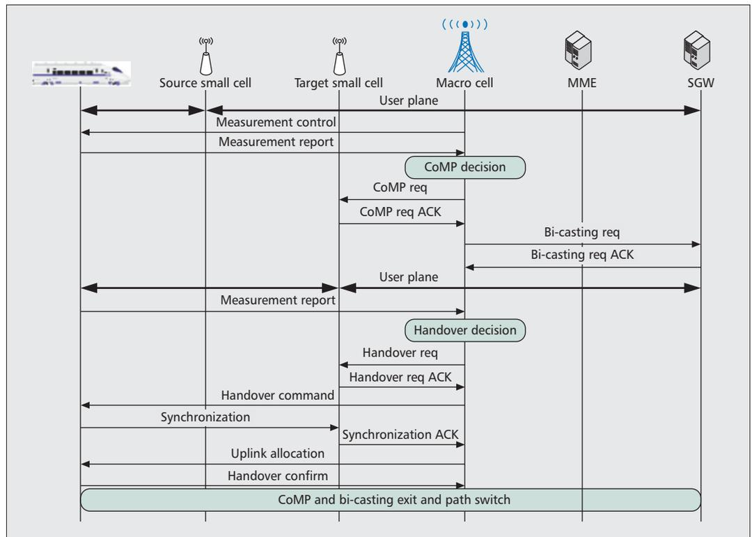
Figure 2. CoMP and Bi-casting based U-plane handover process.
