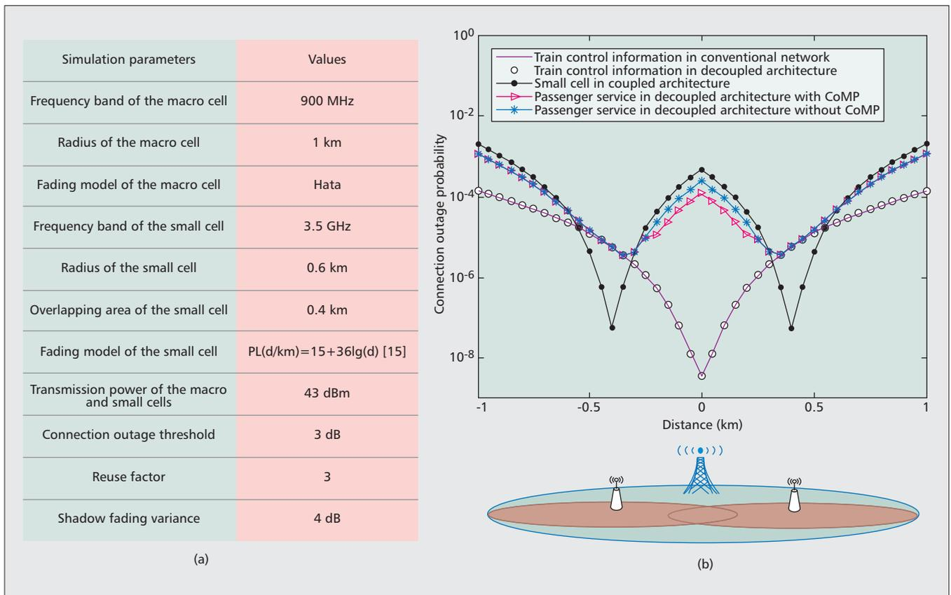
Figure 5. The connection outage probability comparison.
