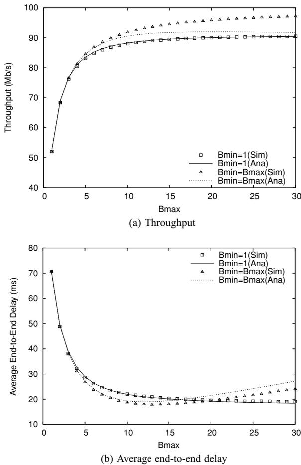
**Fig. 8** Performance versus  $B_{max}$  ( $N = 10$ ,  $T_{sync} = 10 \mu s$ ,  $R = 100$  Mb/s)
