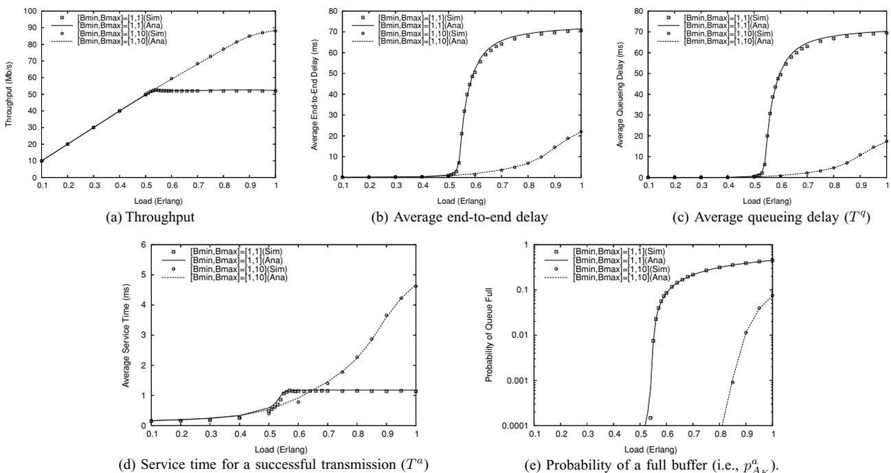
**Fig. 5** Performance versus incoming traffic load ( $N = 10$ ,  $T_{\text{sync}} = 10 \mu\text{s}$ ,  $R = 100 \text{ Mb/s}$ )
