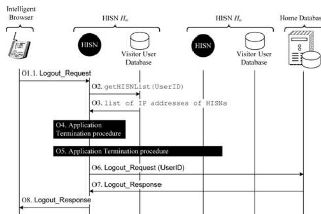
Fig. 12 The message flow for the Logout procedure
