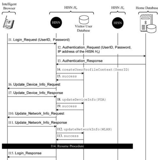
**Fig. 7** The message flow for the Login procedure
