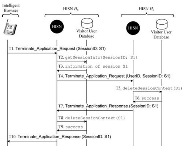
Fig. 11 The message flow for the Application Termination procedure
