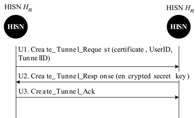
**Fig. 10** The message flow for the tunneling procedure
