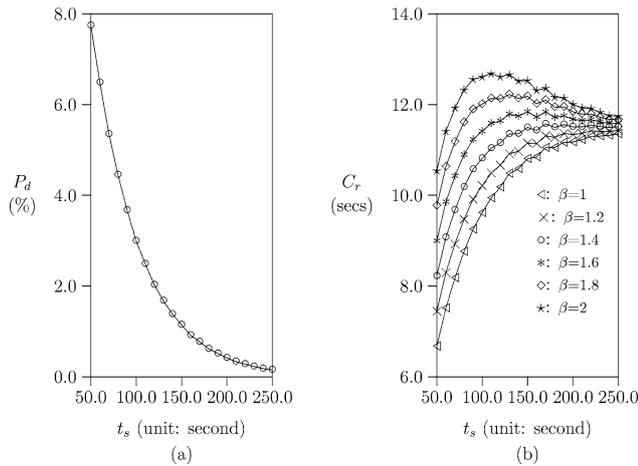
**Fig. 13** Effects of  $T_s$  setup for FTP sessions ( $\frac{1}{\mu_h} = 50$  secs;  $\frac{1}{\mu_l} = 1$  sec;  $\frac{1}{\mu_r} = 1$  sec;  $\frac{1}{\eta_a} = 900$  secs;  $\alpha = 4$ ;  $\frac{1}{\mu_F} = 429$  secs;  $t_a = 1800$  secs)
