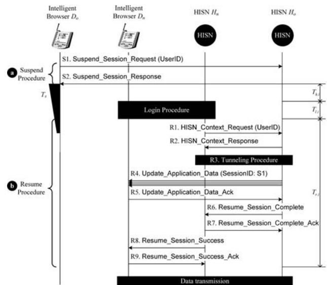
**Fig. 9** The message flow for the suspend and resume procedures
