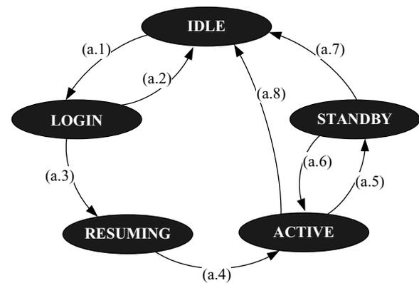
**Fig. 5** State diagram for state machine  $S_u$  for user behavior
