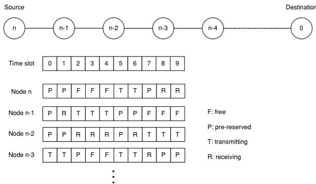
Fig. 2 Example of pre-reservation failure
