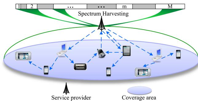
Fig. 1. The architecture of a multi-radio multi-channel multi-hop cognitive cellular network ( $M^3C^2N$ ).
