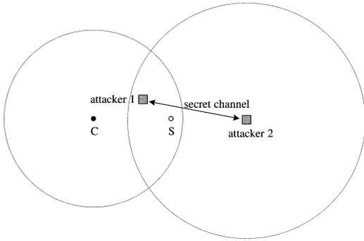
Fig. 2. Topology of an exemplary distance enlargement attack.
