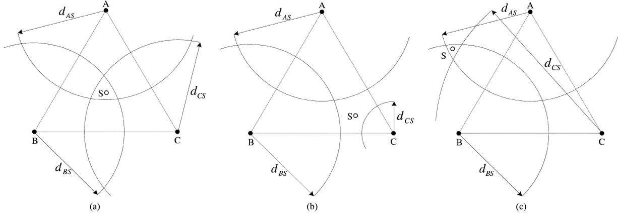
Fig. 1. An exemplary two-way ToA localization process, where anchors  $A$ ,  $B$ , and  $C$  are determining the location of sensor  $S$ . (a) No attacks. (b)  $d_{CS}$  is reduced. (c)  $d_{CS}$  is enlarged.
