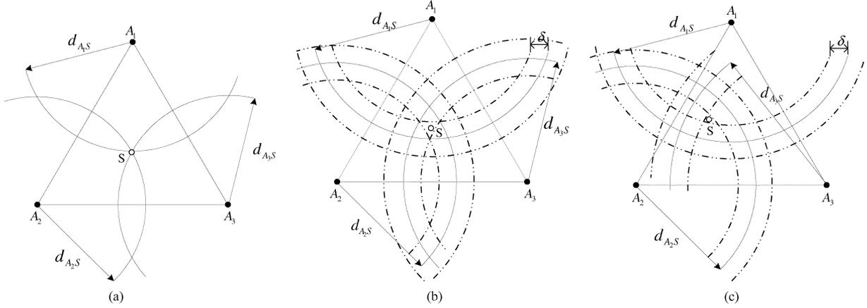
Fig. 4. Location validity test with three anchors. (a) No measurement errors. (b) Measurement errors exist. (c)  $d_{A_3S}$  is enlarged.
