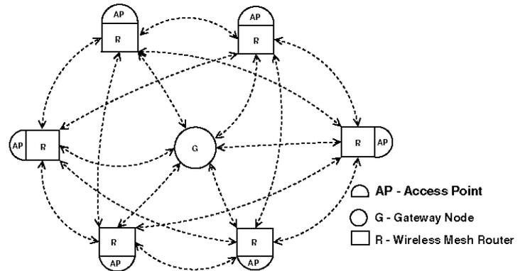
Fig. 1. Hierarchical structure of wireless mesh access networks.
