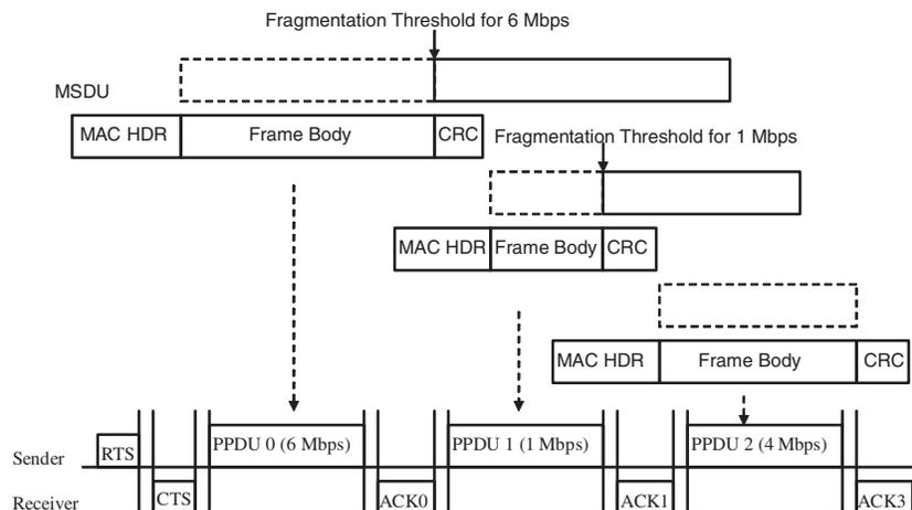
FIGURE 15.10 Dynamic fragmentation process and the timeline of data transmission.
