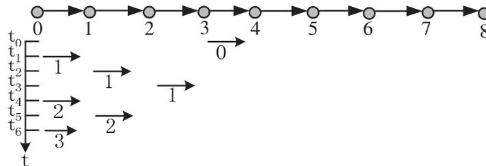
FIGURE 15.8 Packet scheduling when congestion occurs at node 4. The congestion can result from interference or contention from any crossing flow such that node 4 cannot grab the channel in time.
