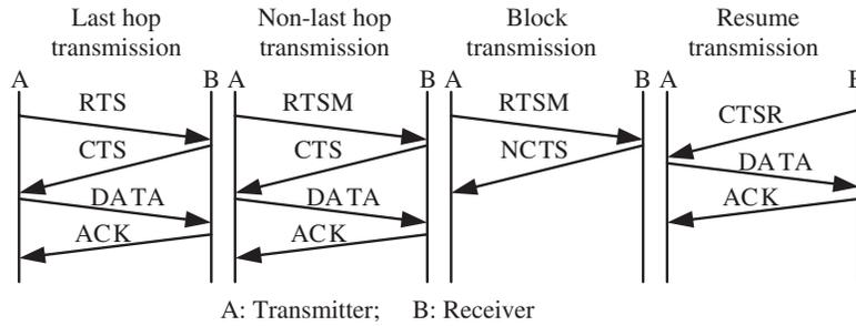
FIGURE 15.7 Message sequence for packet transmission.
