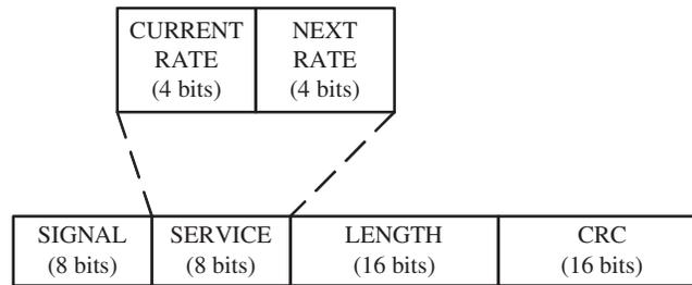
FIGURE 15.11 Physical layer header format in the proposed protocol.
