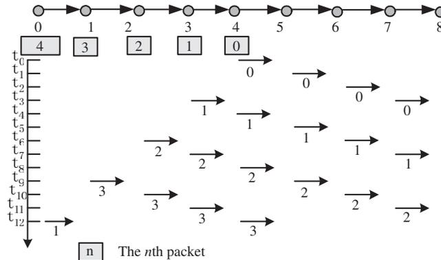
**FIGURE 15.9** Packet scheduling after eliminating the congestion at node 4. After backward-pressure scheduling takes effect, the upstream nodes of this flow and all other crossing flows yield the transmission opportunity to the congested node. Thus, node 4 can quickly forward the backlogged packets and hence the congestion is eliminated.
