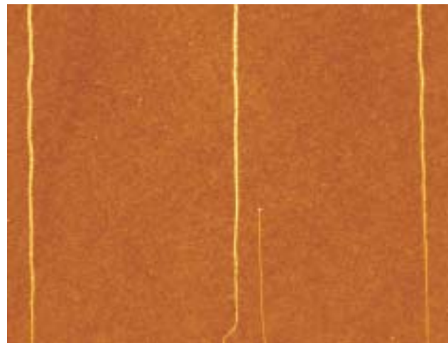
Atomic force microscopy image of 10-microns-long single-walled carbon nanotubes (yellow color) on oxide aligned by an electric field applied in situ during chemical vapor deposition growth.
