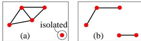
Figure 2: Illustration of the difference between isolated node and disconnectedness. (a){There exists isolated node}  $\Rightarrow$  {The network is disconnected}; (b){the network is disconnected}  $\not\Rightarrow$  {There exists isolated node}.
