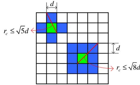
Figure 1: Construction of the percolation model. We divide the plane in squares of size  $d \times d$ . By setting the relation between  $r_c$  and  $d$ , we can make sure that any pair of nodes located in two “neighbor” squares are connected.
