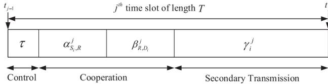
Fig. 3. Multi-phase time slot of a SU.
