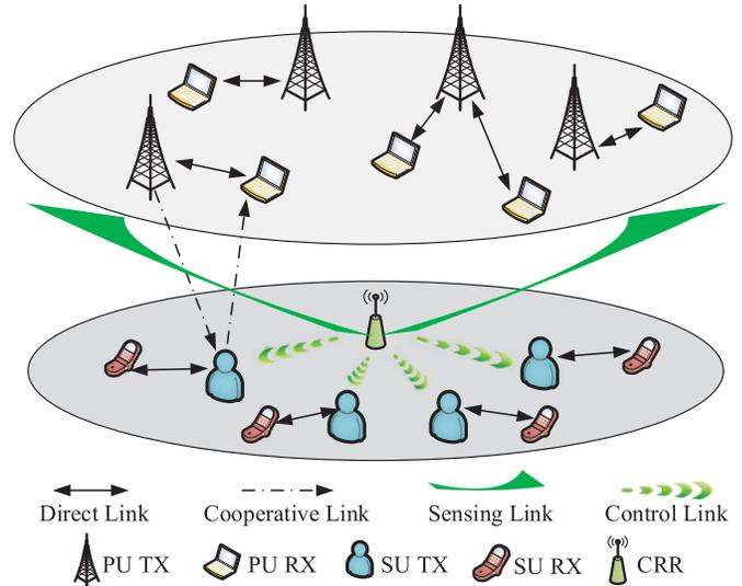
Fig. 2. Network topology of a CCRN.
